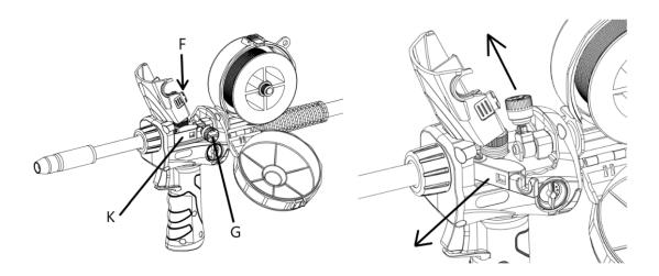
**Step 5:** Feed the free end of the wire through the wire feed mechanism until it enters the inlet guide of the torch neck.
