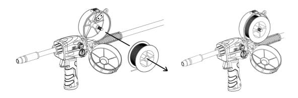
**Step 4:** Press in on the Mechanism Cover Release (F) to open the cover. Rotate the cover all the way forward out of the way. Rotate the Wire Tension Adjustment Knob (G) counterclockwise to unlock the tension mechanism. Rotate the entire Wire Tension Adjustment Knob armature upward to release the Idler Arm (K).
