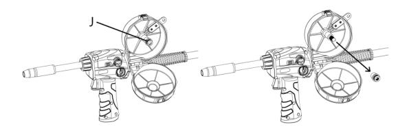
**Step 3:** Install the spool of wire on the main shaft ensuring that the wire is feeding from the bottom of the spool. Insert the free end of the wire into the wire inlet guide at the base of the spool compartment. Re-install Wire Spool Retention Nut (J).
